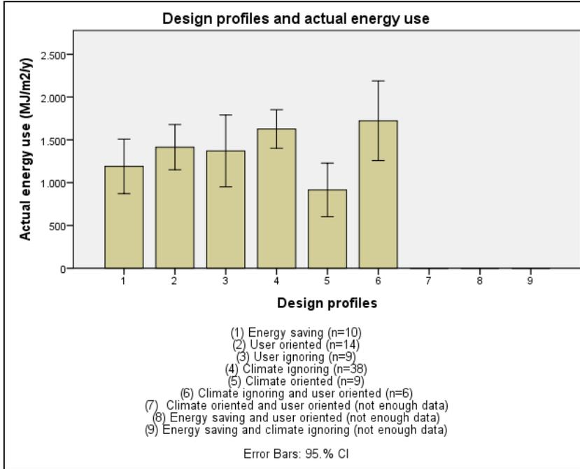
Figure 1 : Influence of the design profiles on the energy use indicator
