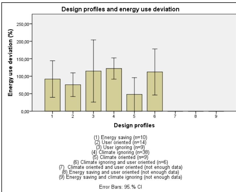
Figure 2 : Influence of the design profiles on the energy use deviation indicator
