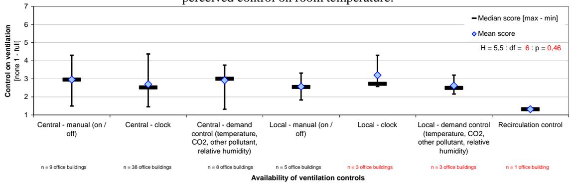
Figure 2. Availability of ventilation controls versus perceived control on ventilation.
