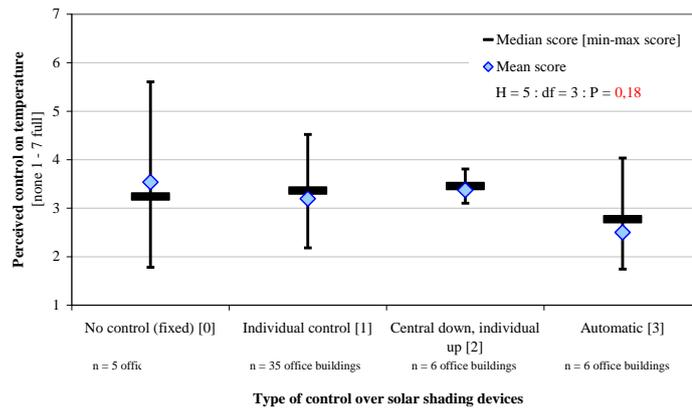
Figure 5. Availability of solar shading devices (no control, individual control, central up individual down, automatic) versus perceived control on room temperature.
