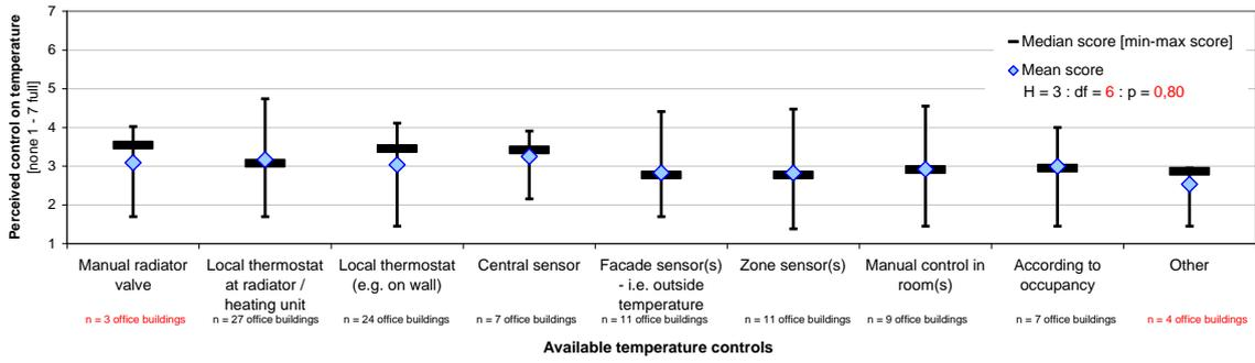
Figure 1. Availability of temperature controls versus perceived control on room temperature.
