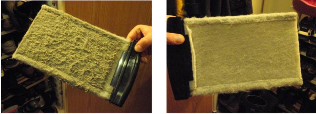
Figure 4: Before and after photos of clogged up MVHR filter following cleaning
