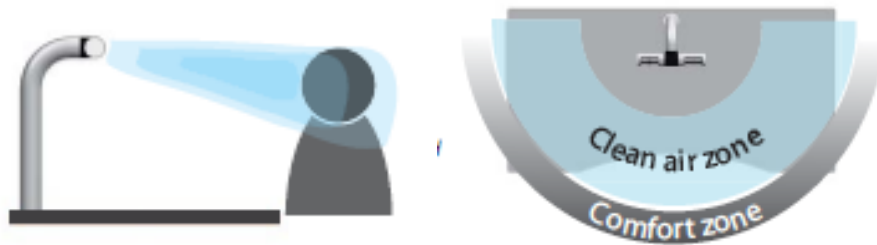
Figure 2: Typical set-up of personalized ventilation system.
