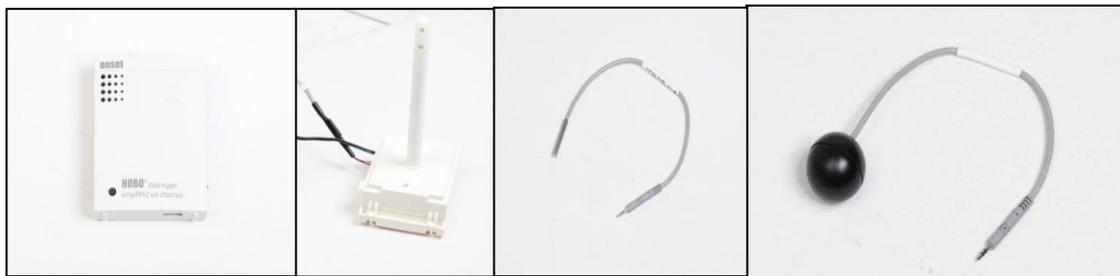
Fig. 3 HOBO logger, Kimo CTV100 air velocity sensor attached to the cable adapter, TMC1-HD thermo sensor and the same thermo sensor attached to black 40mm ping pong ball
