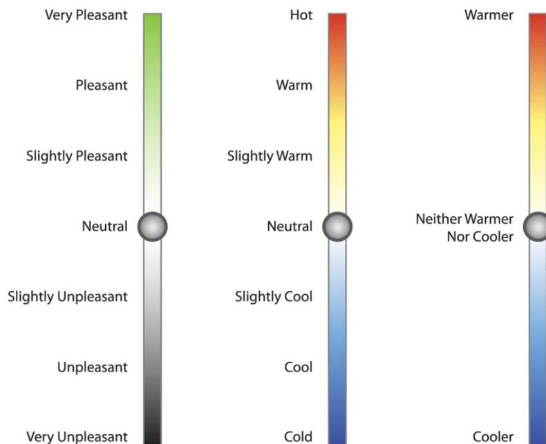
**Figure 2.** Scales of thermal pleasure, thermal sensation, and thermal preference as they appear in the iPad application.
