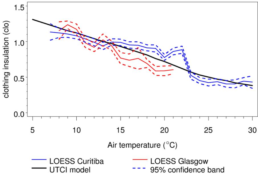
**Figure 3:** Clothing thermal insulation related to air temperature for the samples from Curitiba and Glasgow against predicted (UTCI) clothing insulation
