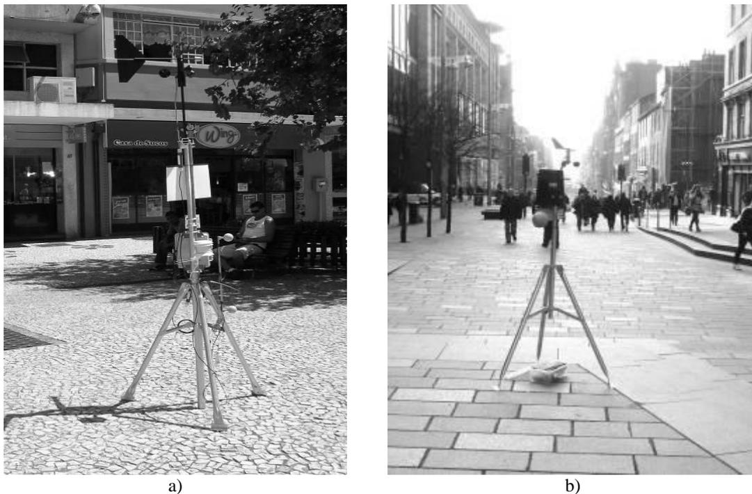
**Figure 1:** Equipment used for microclimatic measurements: a) in Curitiba; b) in Glasgow
