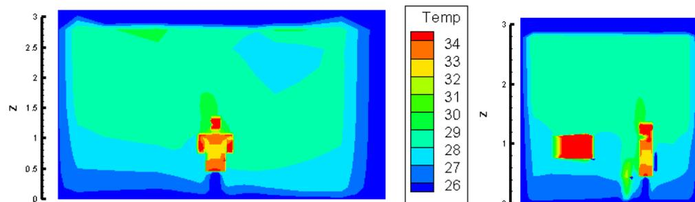
**Figure 7.** Air temperature distribution around the human body for Case 3 (panel at 19°C occupying 80% of ceiling area).
