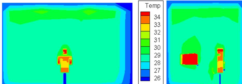
**Figure 5.** Air temperature distribution around the human body (situation without radiant cooling system).
