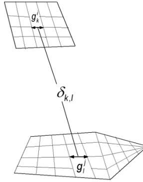
**Figure 2.** Schematic representation of the application of Stokes' theorem to the elementary surfaces.
