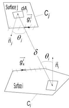
**Figure 1.** View factor associated with radiation exchange between surfaces  $i$  and  $j$ .
