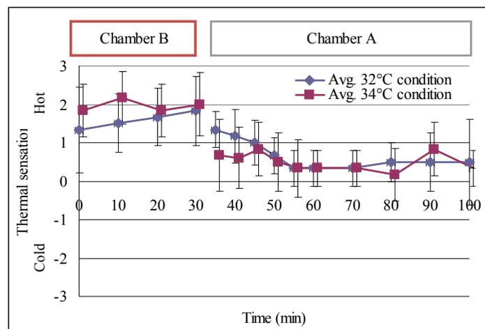
Fig. 3 Temporal change in thermal sensation
