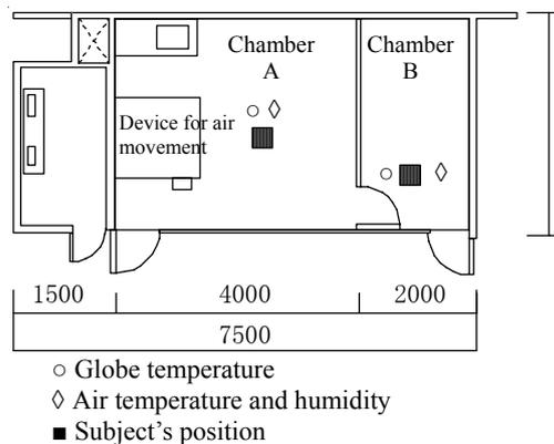
Fig. 1 Test chamber
