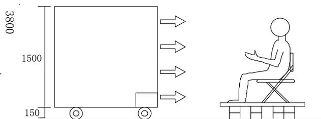
Fig. 2 Device for uniform air movement and sitting conditions for the subject
