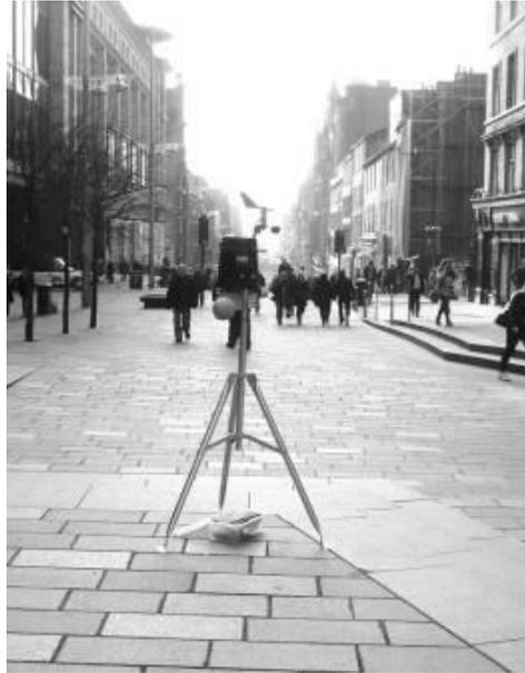
**Figure 2.** ‘Mobile’ weather station (Davis Vantage Pro2) with gray globe thermometer.
