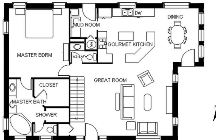
**Figure 2.1: 2,400 ft<sup>2</sup> Typical House Floor 1**
