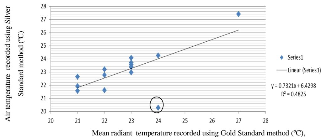
Figure 10: A regression of air temperature measured using the Silver Standard method vs. mean radiant temperature measured using the Gold Standard method (includes data from all 16 houses).
