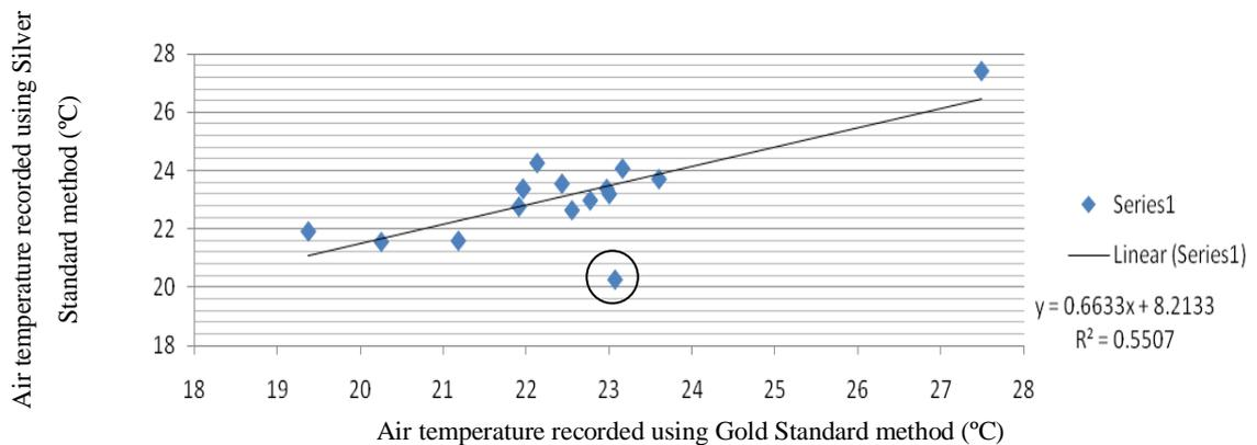
Figure 6: A regression of indoor air temperature measured using the Silver Standard method vs. indoor air temperature measured using the Gold Standard method (includes data from all 16 houses).
