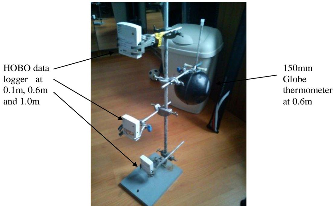
Figure 5: Detailed view of the equipment setup for the Gold Standard method
