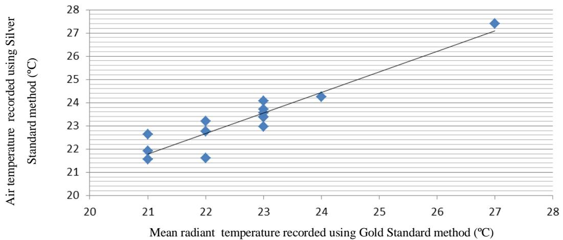
Figure 11: A regression of air temperature measured using the Silver Standard method vs. mean radiant temperature measured using the Gold Standard method (house no.6 data excluded).
