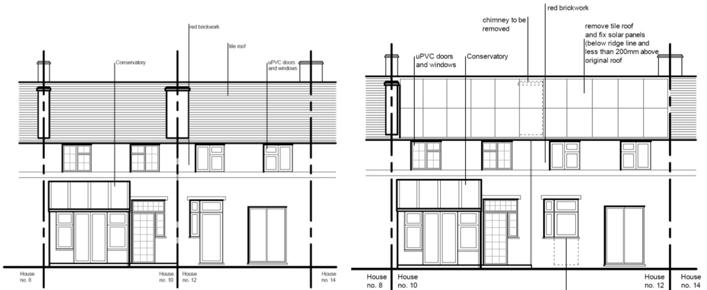
Figures 3 and 4 - initial survey and proposal for solar panels to fully cover the rear roof to nos 10 and 12 Laneway - Rear elevation
