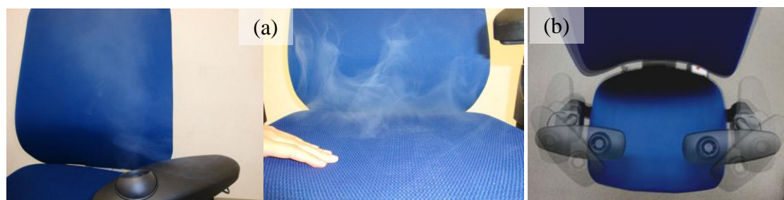
Fig. 2. (a) Airflow from the armrest and the seat; (b) Range of motion of the armrests
