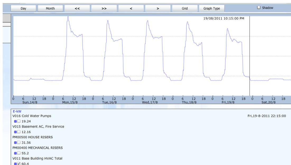
Figure 6: Reduction in Heating, Ventilation and Air Conditioning (HVAC) sub-meter morning ‘spike’ at Building A1 indicating a reduction in space temperature setpoint reduced heating / cooling conflicts.
