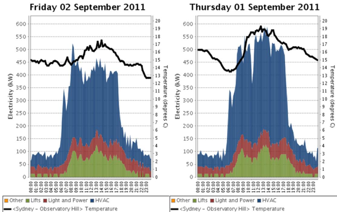
Figure 8: Impact of annual chiller service at Building A1. Chillers were 'locked out' on Friday 2 Sept. and a 23% saving was reported with no 'too hot' complaints. (Graphic sourced from 'Pulse' message.)
