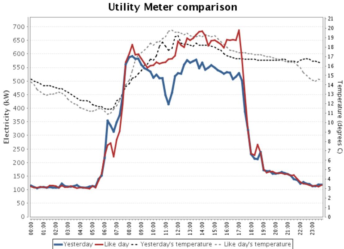
Figure 7: Impact of fine-tuning temperature setpoints at Building A1, 31 Aug, 2011. (Graphic sourced from 'Pulse' message.)
