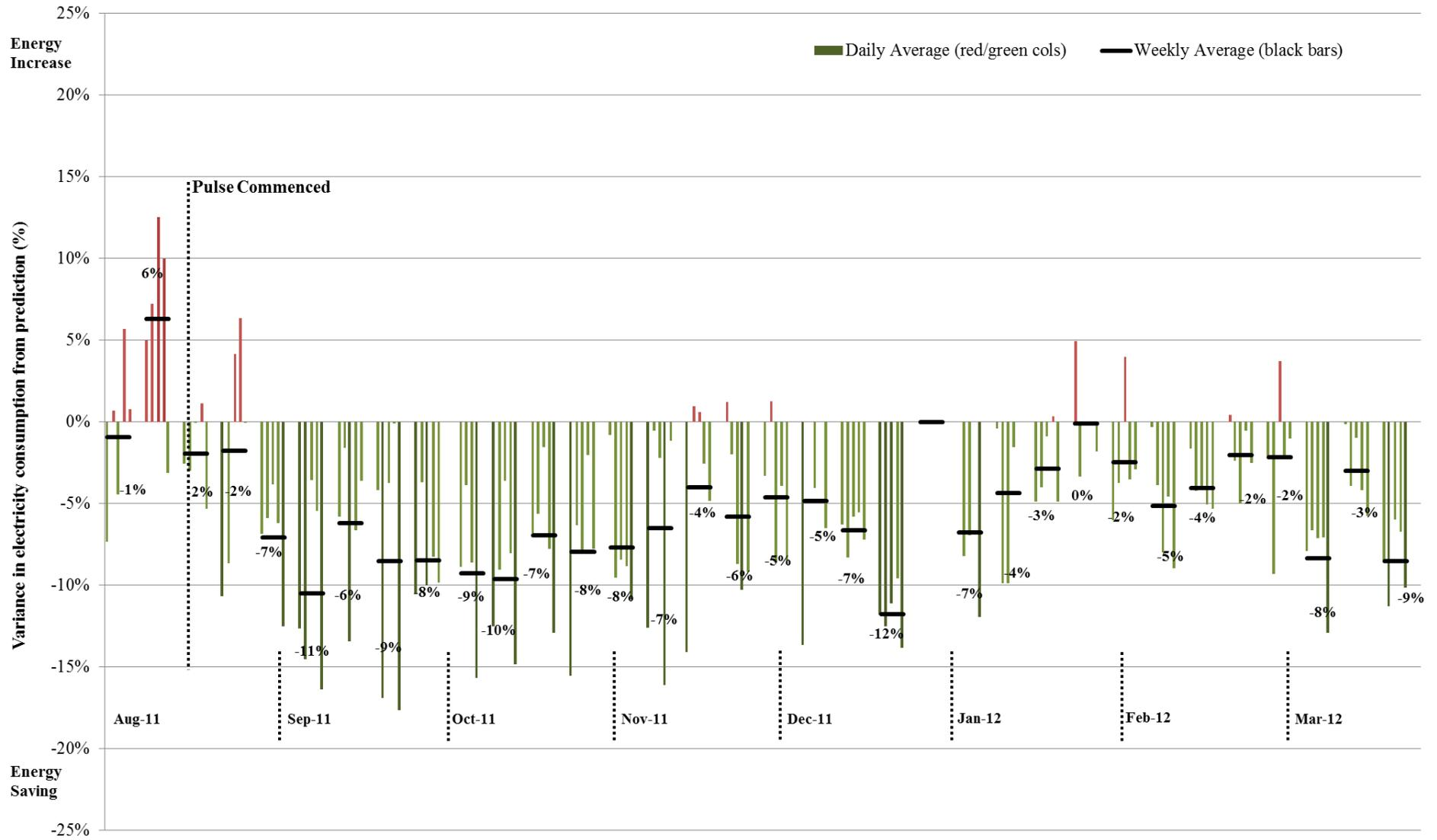
Figure 4: Mean daily and weekly variance between actual and predicted electricity use for the three buildings in Group A, from two weeks prior to commencement.
