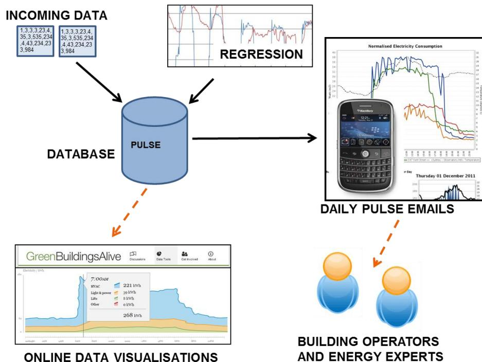
Figure 2: Overview of 'Pulse' system architecture.
