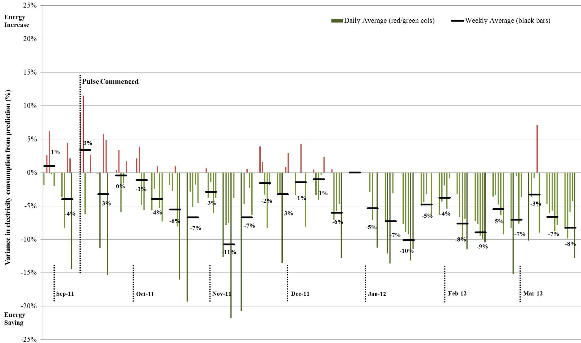
Figure 5: Mean daily and weekly variance between actual and predicted electricity use for the four buildings in Group B, from two weeks prior to commencement.
