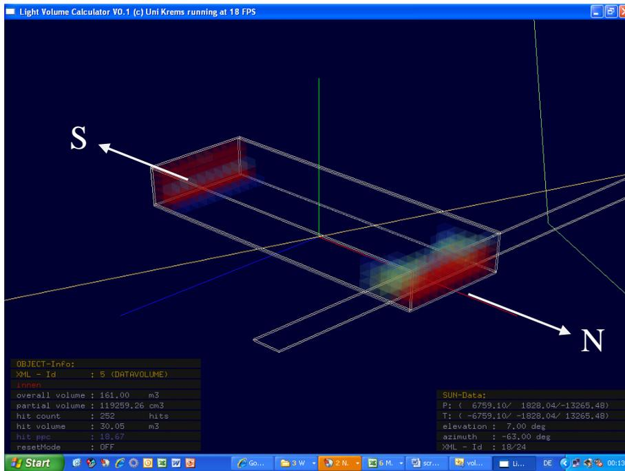
**Figure 5: Perspective Visualization of a daily LPF calculation, valid for June 21<sup>st</sup> at Vienna**
