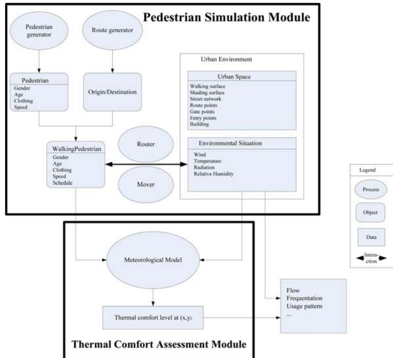
Figure 1: Software structure of the computational system.
