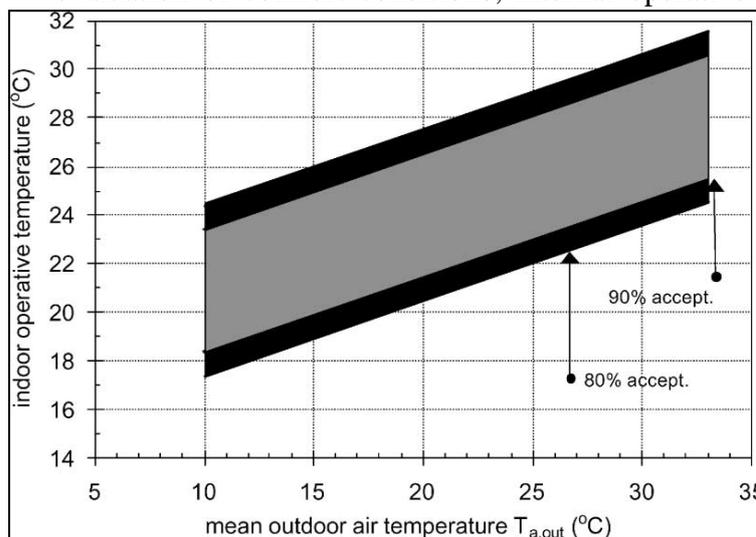
Figure 3. Acceptable operative temperature ranges for naturally conditioned spaces according to ASHRAE 55 (from ASHRAE Standard 55)
