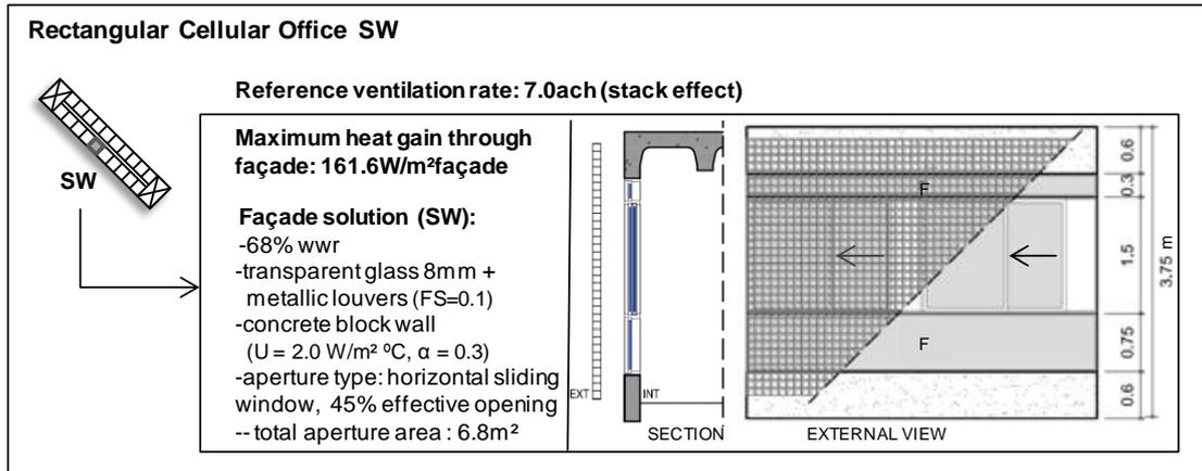
Figure 8. Possible solutions for the northeast and the southwest façades of the rectangular open plan office building, under wind effect ventilation – SOLUTION 2 and SOLUTION 3, respectively
