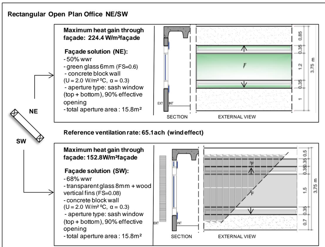
In all three cases the users have control of the windows and therefore can adjust the ventilation conditions of the offices.
