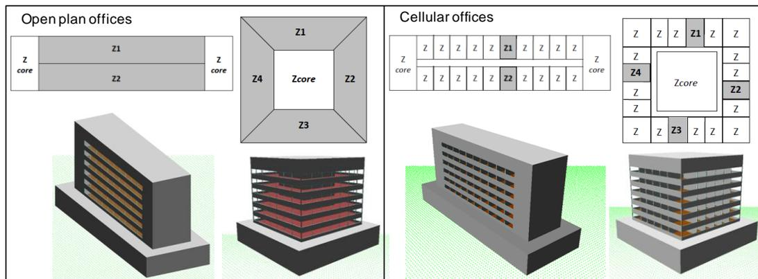
Figure 6. Rectangular and square building models at TAS: plans with zones of analysis and building external views; open plan offices (left) and cellular offices (right).
