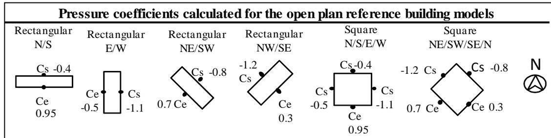
Figure 5. Pressure coefficients for air inlet ( $C_e$ ) and air outlet ( $C_s$ ) calculated for the reference building models according to wind direction, with the method proposed by Sharag-Eldin (2007)
