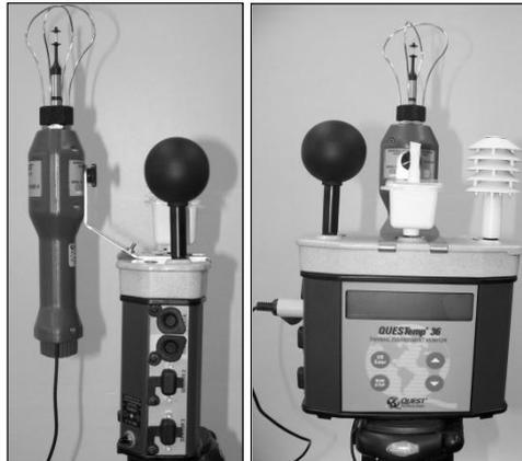
**Figure 3: Monitor of thermal stress**
