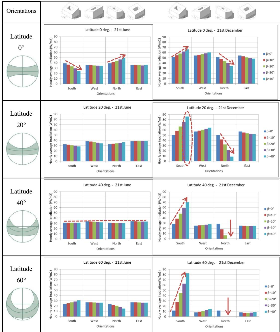
Figure 2. Effects of changing slope of the building's roof on the received irradiation by the courtyard walls in different orientations and latitudes
