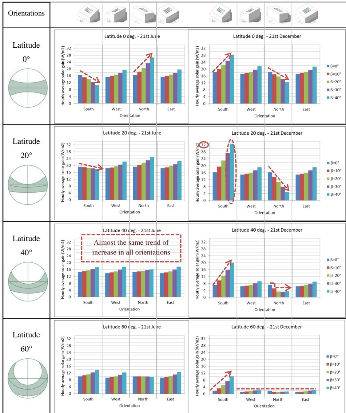
Figure 3. Effects of changing slope of the building's roof on the received irradiation by the internal surfaces of the atrium in different orientations and latitudes
