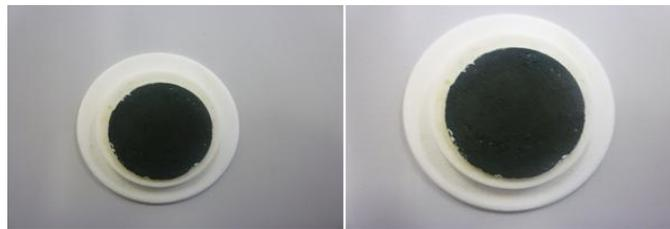
Figure 4. Cathode electrode layer before (left) and after (right) the sintering.
