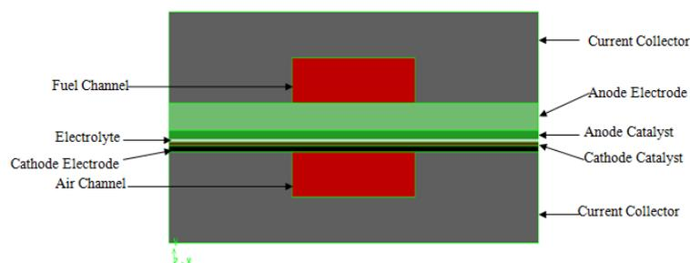
Figure 5. Fuel cell computational model arrangement
