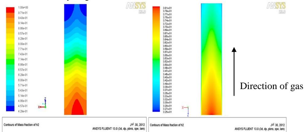
Figure 9. Mass fraction of hydrogen on the anode electrode/catalyst interface (Right: Starck's cell, Left: Designed cell)
