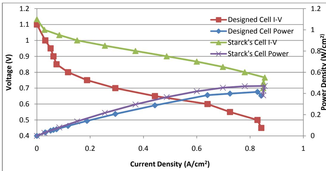
Figure 8. Comparison of the I-V and power curves from the simulation results
