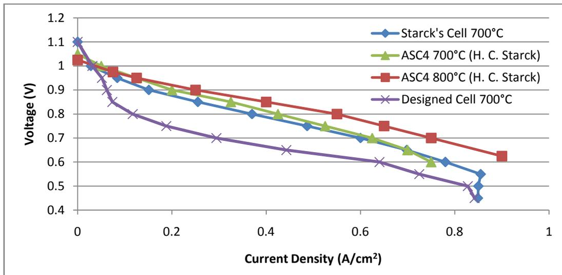
Figure 7. Comparison of the I-V curves from the experimental results and the simulation results
