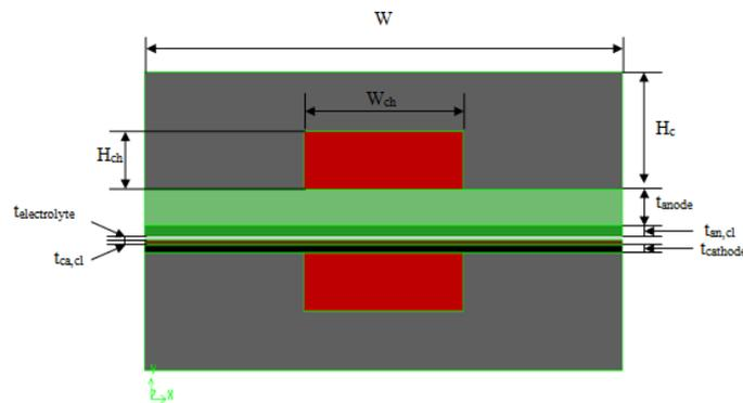
Figure 6. Fuel cell dimensions
