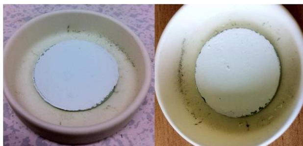
Figure 2. Electrolyte layer before (left) and after (right) the sintering process
