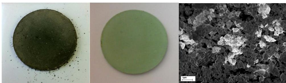
Figure 1. Anode substrate before (left) and after (centre) the sintering process and the SEM picture in 1  $\mu\text{m}$  scale.
