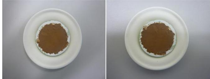
Figure 3. Cathode catalyst layer before (left) and after (right) the sintering.
