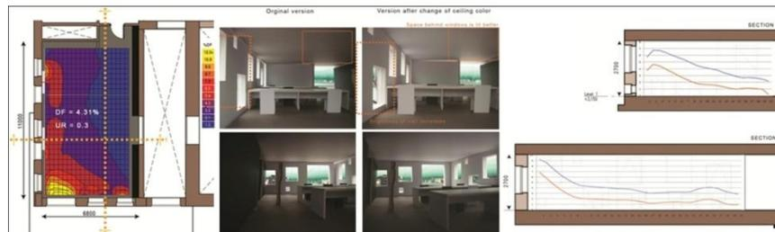
Figure 9 Comparison of daylight distribution between existing case and case after changing reflectance of ceiling
