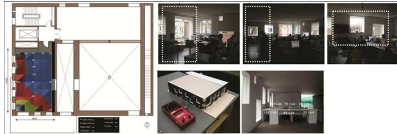
Figure 7 Existing luminous environment of office room and site measurement and physical model in Artificial sky
