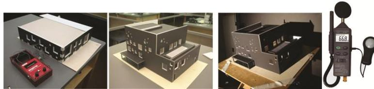
Figure 3 Photographs of the physical model in Artificial Sky and Heliodon testing
