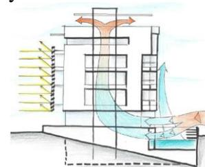
Fig.8 Evaporative cooling combined with stack ventilation through staircase, R C TECH, 2010
