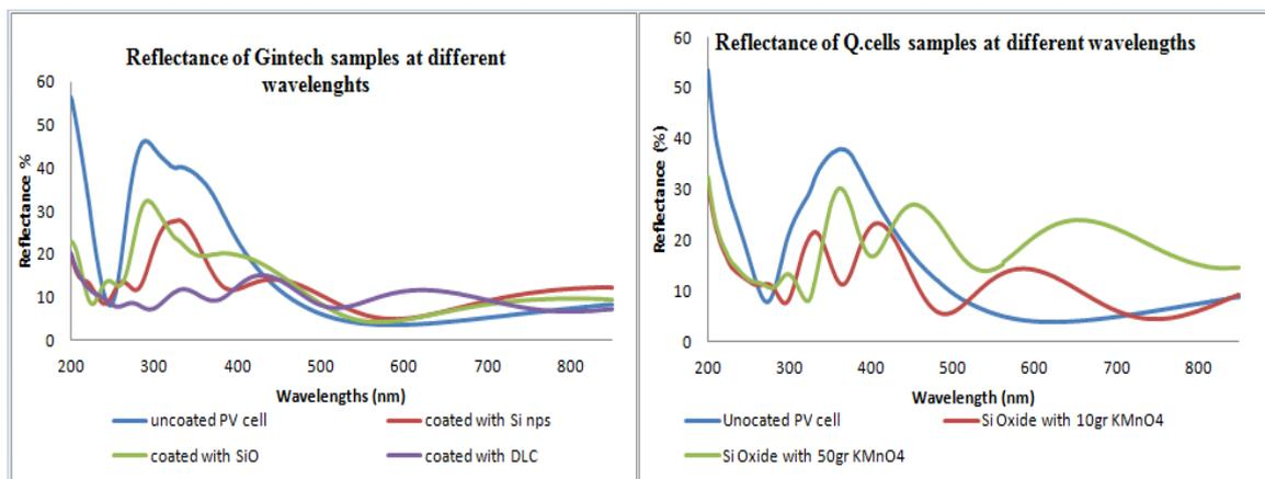
Figure 5: Changes in the reflectance of PV cells before and after coating for Gintech and Q.cells
