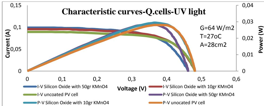
Figure 4: Characteristic curves of Q.cells multicrystalline PV cells under UV light
