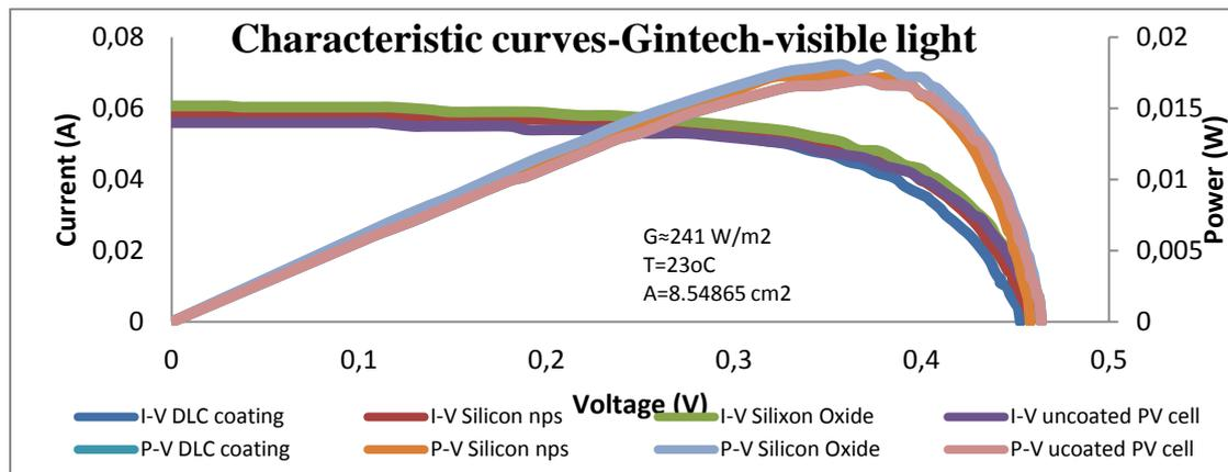
Figure 1: Characteristic curves of Gintech polycrystalline PV cells before and after coating under visible light
