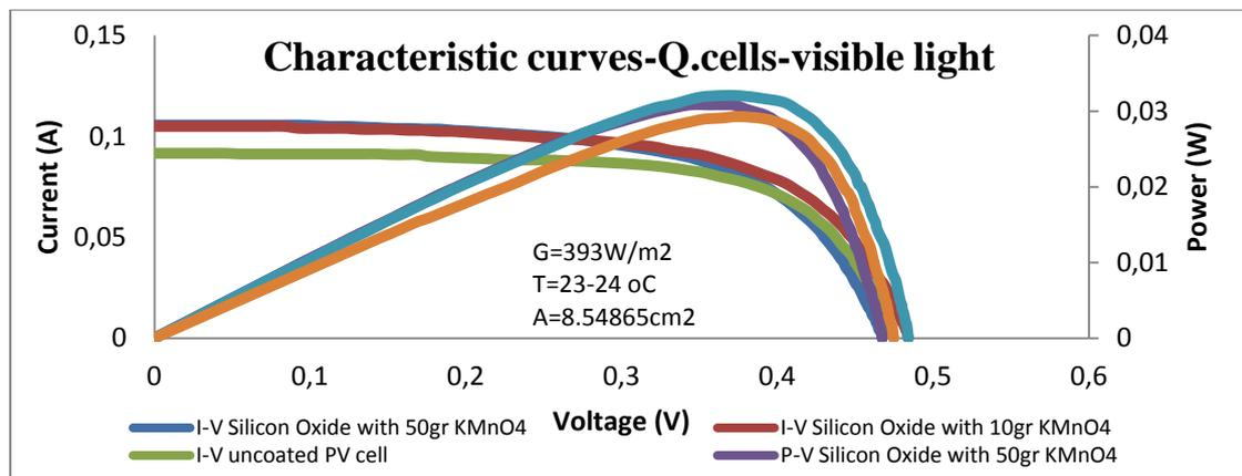
Figure 3: Characteristic curves of Q.cells multicrystalline PV cells under visible light
