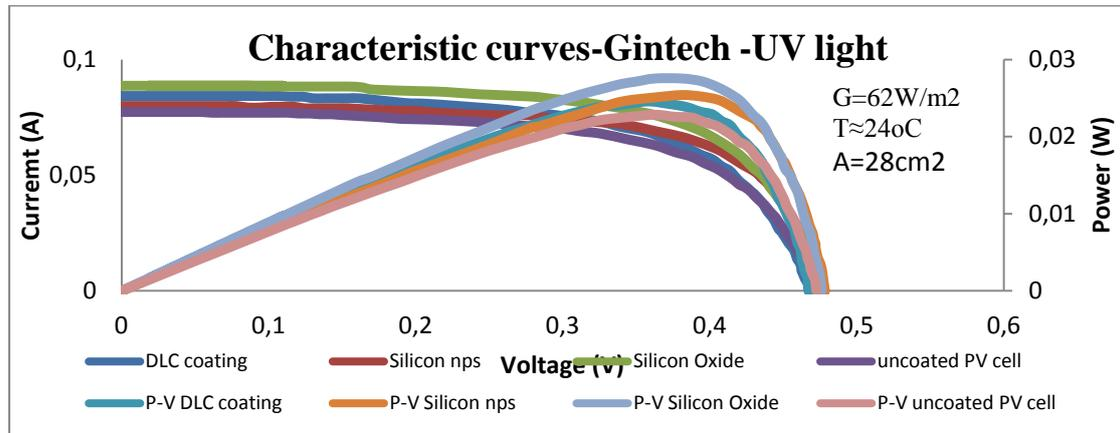
Figure 2: Characteristic curves of Gintech polycrystalline PV cells under UV light
