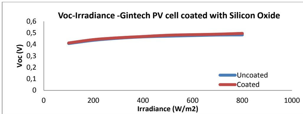
Figure 6: Open circuit voltage dependence from solar irradiance for the Gintech polycrystalline PV cell
