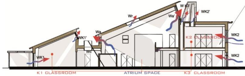
Figure 3: Natural ventilation in section- inlets and outlets (drawn by author)
