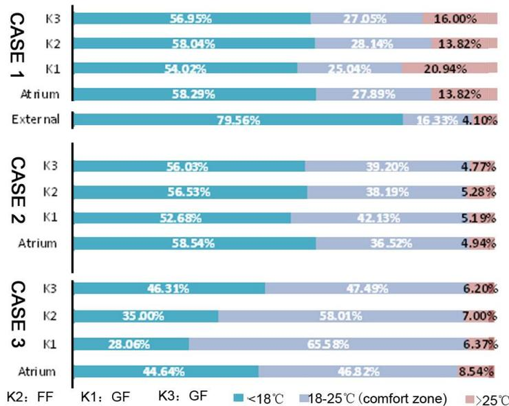
Figure 4: Annual proportion of hours for different temperature range in school hours of winter and summer to access the cooling efficiency for the internal gains, containing the occupants, lighting, equipment
