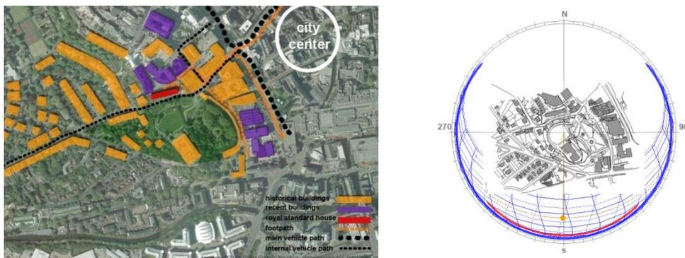
Figure 2: Site analysis (on the left hand side) and sun-path diagram (on the right hand side) for Royal Standard House
