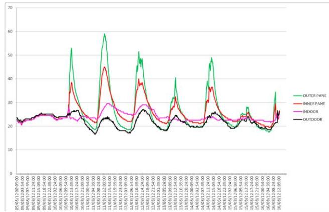
Figure 3 Temperatures graph south facade
