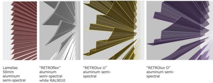
Figure 3. Typical lamellas 50mm and the 3 Köster systems.
