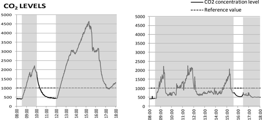
Fig. 3 & 4. CO<sub>2</sub> concentration values in room A.11 on February 11<sup>th</sup> and May 27<sup>th</sup> 2010
