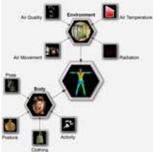
Figure 3: Factors to predict thermal comfort experience according to Fangers model.
