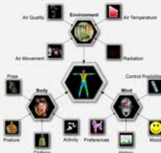
Figure 6: Factors to predict thermal comfort experience according to the adaptive model
