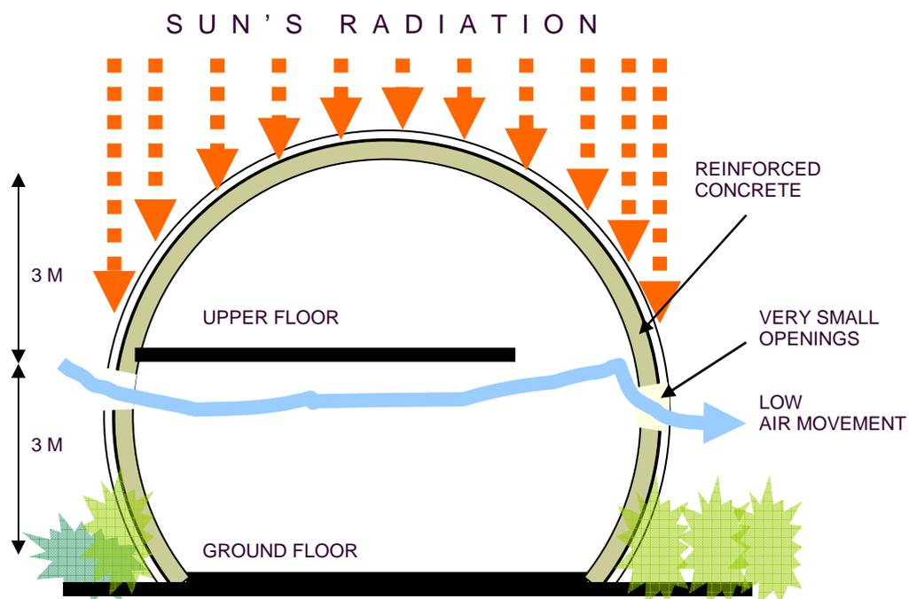
Figure 2. Section of Nglepen dome shelters
