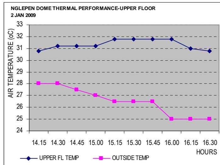
Figure 5. Nglepen dome shelter – Upper floor temperature performance (centre)
