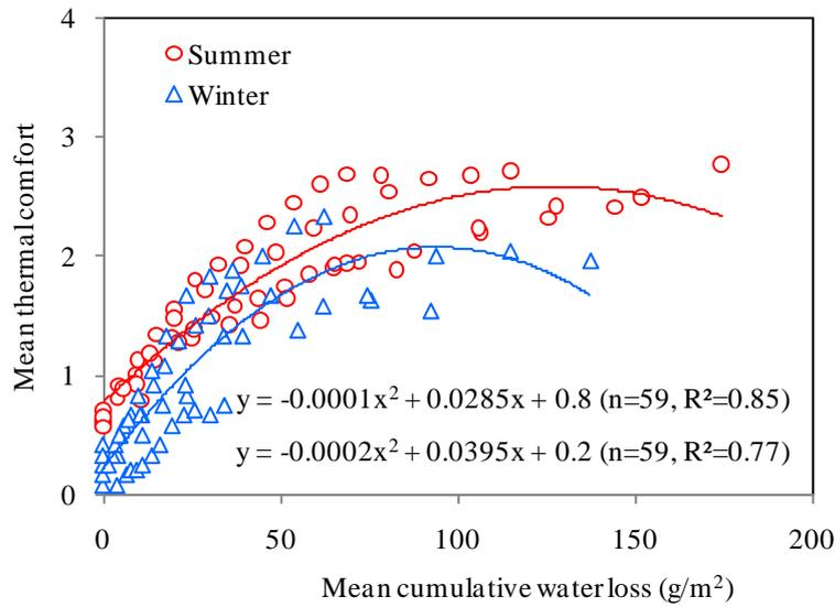
**Fig. 18.** Relationship between thermal comfort and cumulative water loss. The data was averaged for each case and voting time. Each point includes 12 to 27 data readings. All regression coefficients or correlation coefficients are significant ( $p < 0.001$ ).
