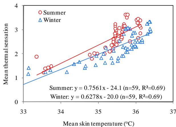
**Fig. 12.** Relationship between thermal sensation and skin temperature. Each point includes 12 to 27 data readings. All regression coefficients or correlation coefficients are significant ( $p < 0.001$ ).
