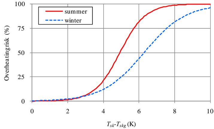
**Fig. 16.** Proportion of subjects voting ‘uncomfortable’, ‘very uncomfortable’, or ‘extremely uncomfortable’ on the thermal comfort scale (overheating risk) as a function of the difference between the actual and comfortable skin temperatures.
