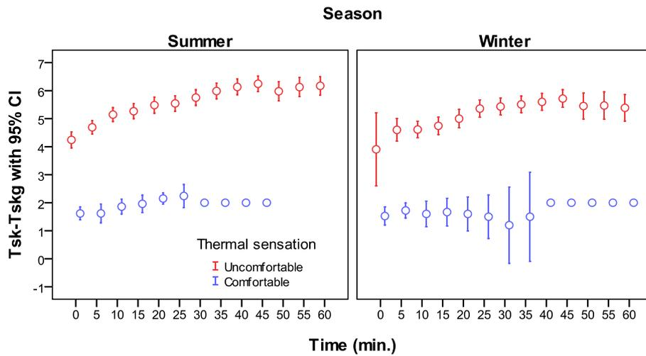
**Fig. 15.** Difference between actual and comfortable skin temperatures ( $T_{sk}-T_{skg}$ ) with 95% confidence intervals during summer and winter experiments. The figure is based on a seven-point thermal sensation scale, counting comfortable as the three central categories. The ‘uncomfortable’ categories are assumed to represent an overheating risk.
