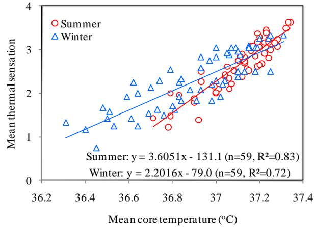
**Fig. 13.** Relationship between thermal sensation and core temperature. Each point includes 12 to 27 data readings. All regression coefficients or correlation coefficients are significant ( $p < 0.001$ ).
