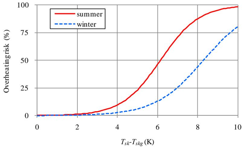
**Fig. 17.** Proportion of subjects voting ‘fairly difficult to tolerate’ or ‘very difficult to tolerate’ or ‘intolerable’ on the thermal tolerance scale (overheating risk) as a function of the difference between the actual and comfortable skin temperatures
