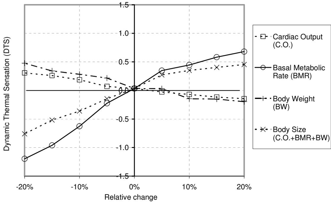
Figure 2. Sensitivity of thermal sensation vote to BMR, C.O. and BW
