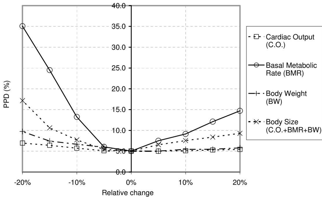
Figure 3. Sensitivity of PPD to BMR, C.O. and BW
