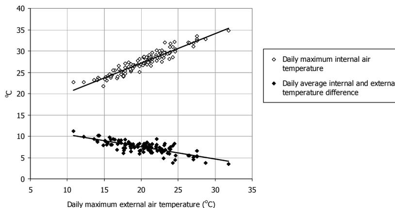
**Figure 5: Simulated internal air temperature results plotted against daily maximum external air temperature using the base-case scenario (2005 climate data, 30% window opening free area and low thermal mass) for the single-sided ventilated classroom in London**
