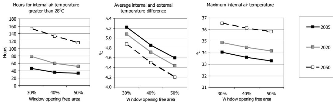
**Figure 6: Simulated internal air temperature results against window free area opening for the cross-ventilated classroom in London using 2005, 2020 and 2050 climate data.**
