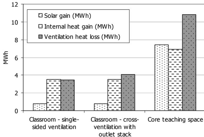
**Figure 4: Total solar gain, internal heat gain and ventilation heat loss (May to September inclusive) for the three simulated teaching spaces using the base-case scenario (2005 climate data, 30% window opening free area and low thermal mass) and London location**
