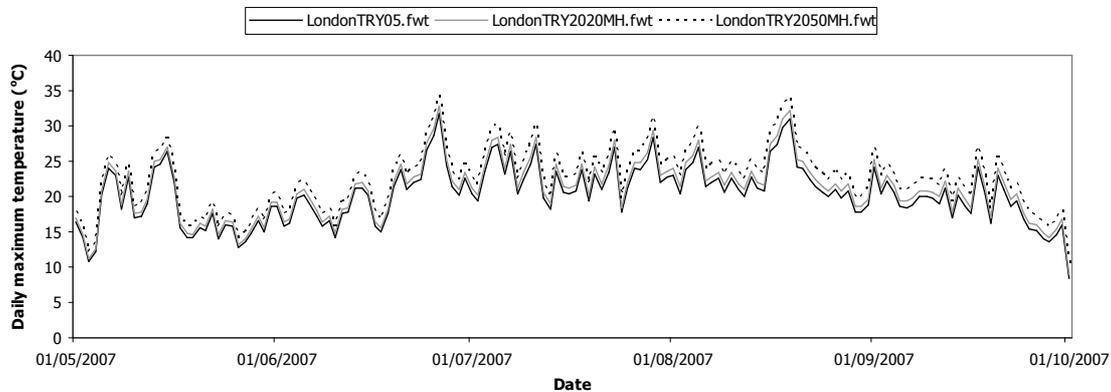
**Figure 3: Daily maximum external air (dry-bulb) temperature for 2005, 2020 medium-high and 2050 medium-high CIBSE Test Reference Year data for London**
