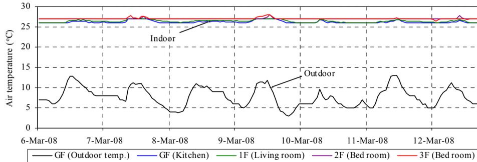
**Fig. 4.** Indoor and outdoor air temperature variation for 7 days.
