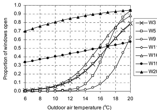
**Fig. 21.** Proportion of window opening as a function of outdoor air temperature in occupied in Autumn.
