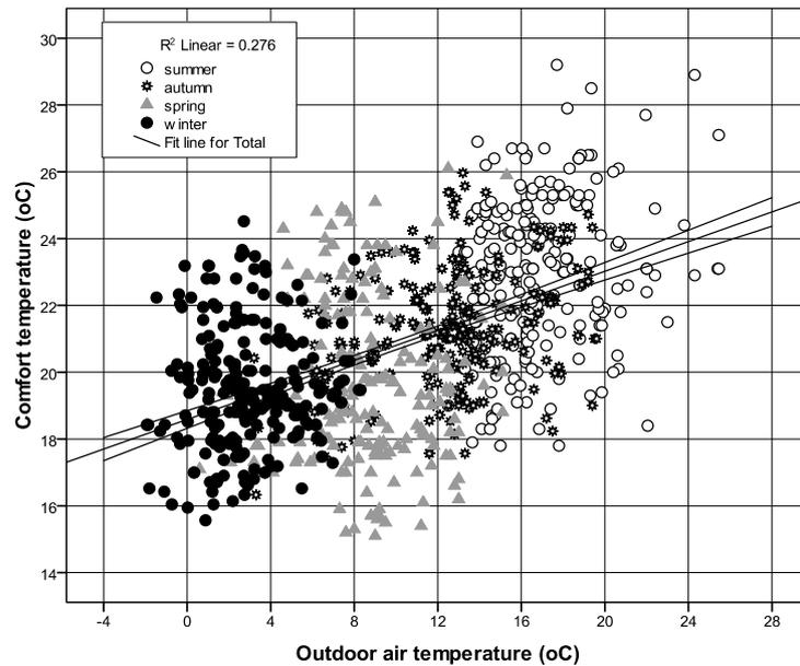
**Fig. 17.** Relation between the comfort temperature and outdoor air temperature.
