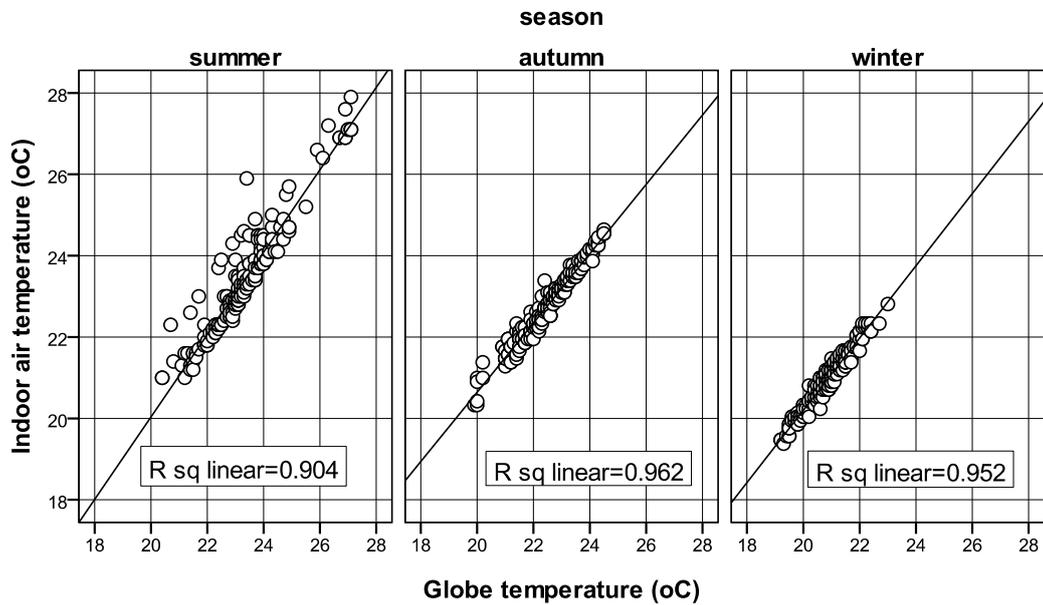
Fig. 15. Relation between the indoor air temperature and globe temperature
