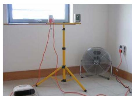
**Fig. 2.** Monitoring equipment set up for the co-heating test
