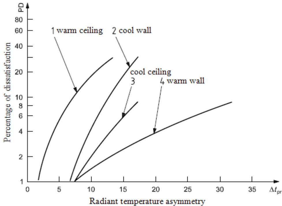
**Figure 6. Local thermal discomfort caused by radiant temperature asymmetry (ISO7730:2005)**
