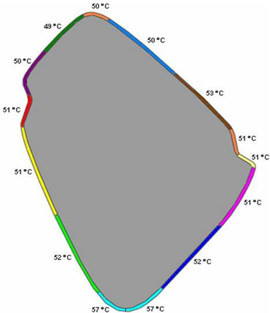
**Figure 13. Air temperature of the 14 sectors with DSF gap being ventilated with 800 l/sec of air from internal spaces**
