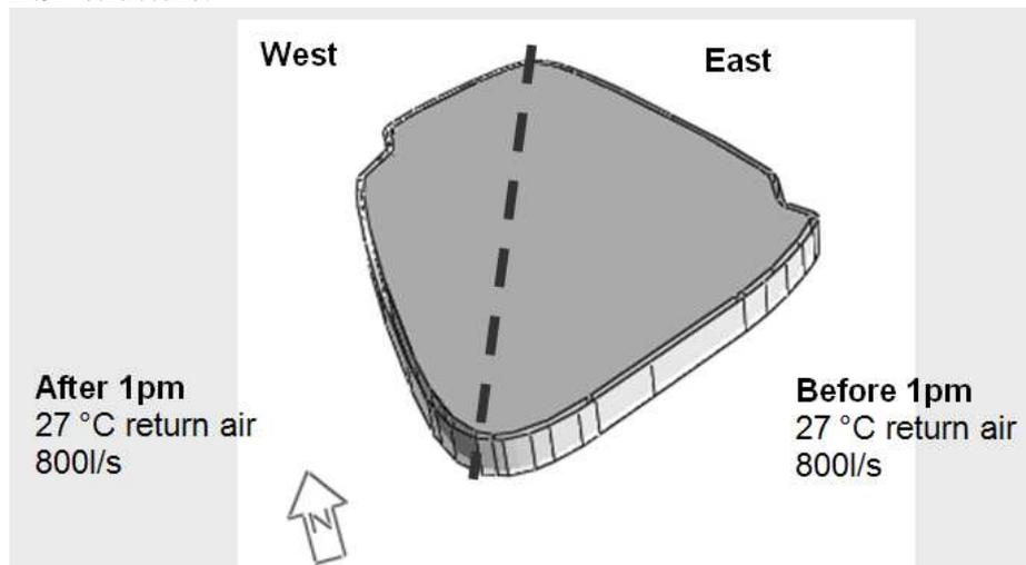
Figure 9. Potential morning and afternoon ventilation flow rate distribution for the Eastern and Western sectors of the DSF gap
