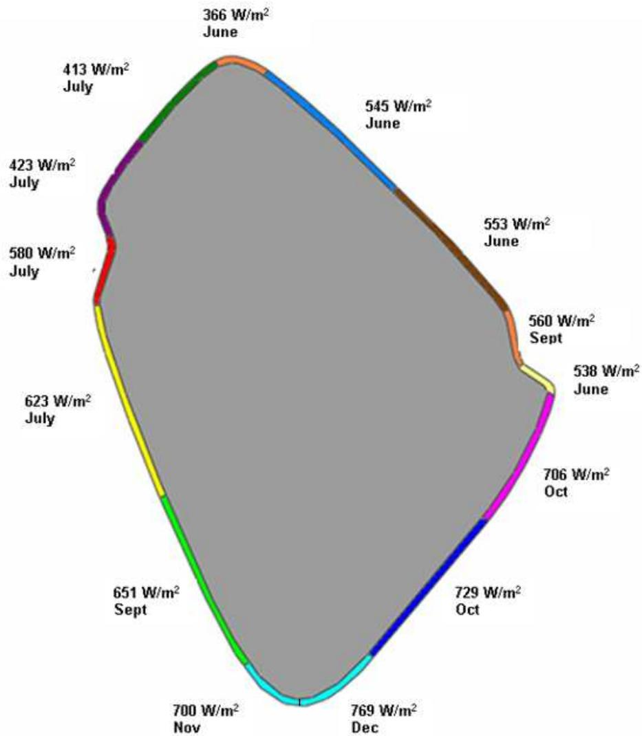
**Figure 7. Incident solar radiation distribution around the perimeter of the façade**
