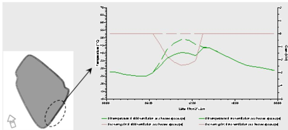
Figure 10. A sample south-eastern façade sector ventilated between 7am and 1pm
