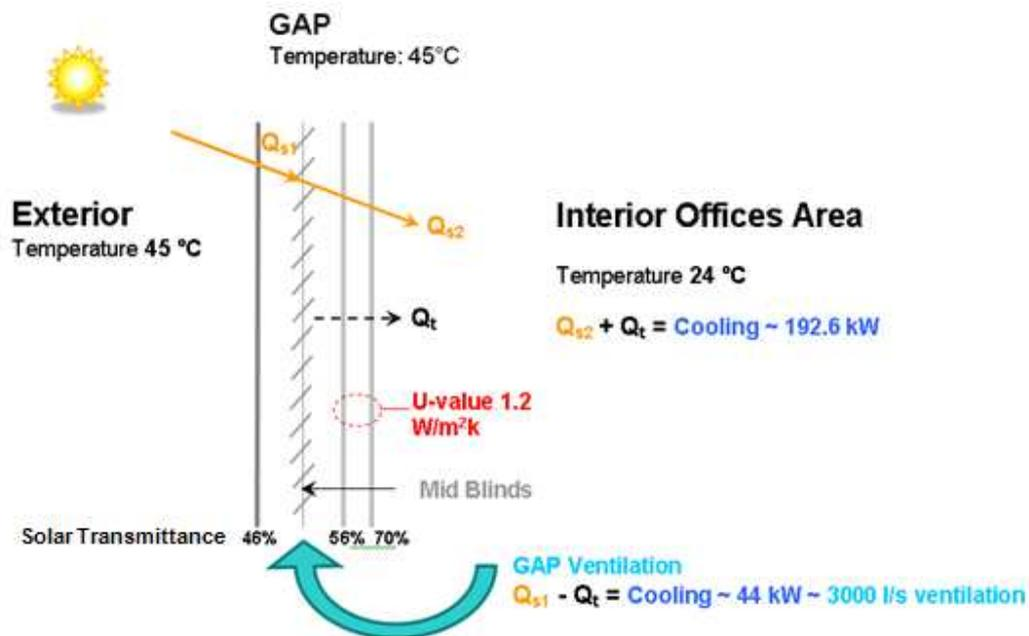
**Figure 3. Cooling requirements when the DSF gap is kept at 45 °C**
