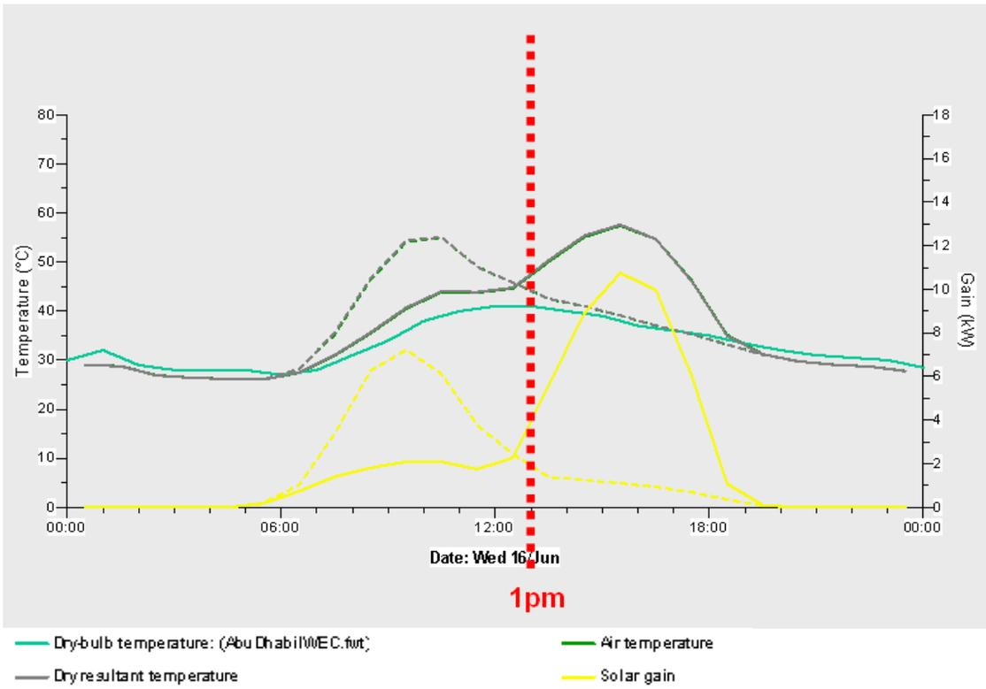
**Figure 12. Temperature variation of ventilated DSF (800 l/sec supplied separately for Eastern and Western zones)**
