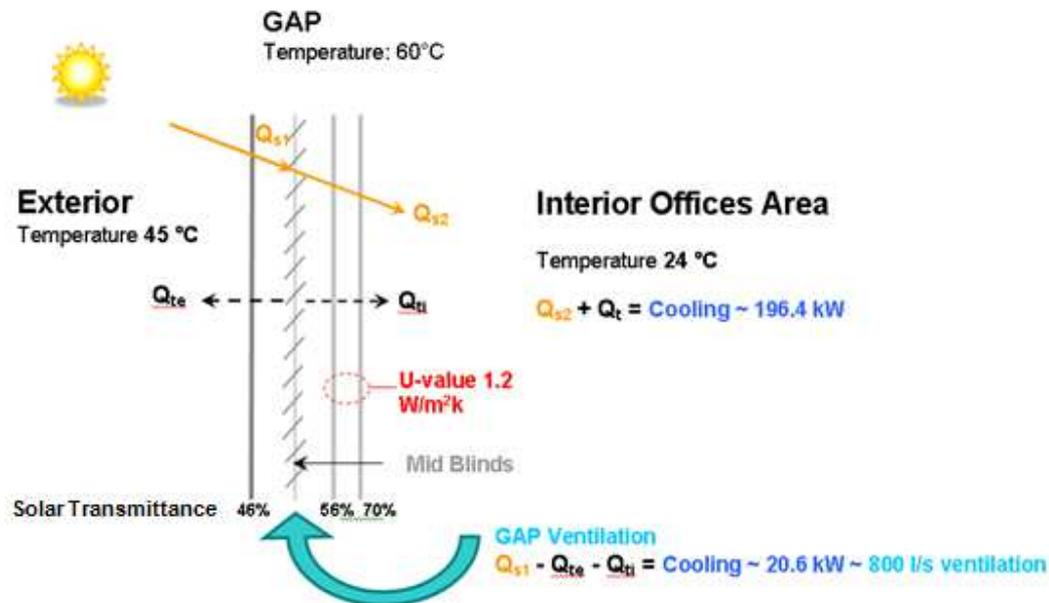
Figure 4. Cooling requirements when the DSF gap is kept at 60 °C
