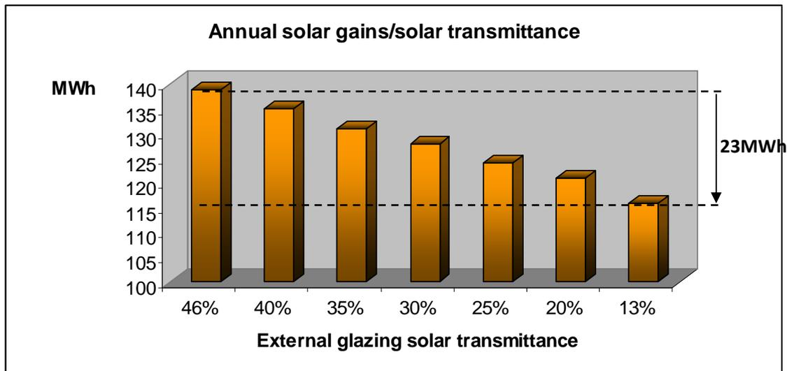
**Figure 14.** Variation of the peak annual solar gains of the selected floor with the solar transmittance of the outer layer external glass
