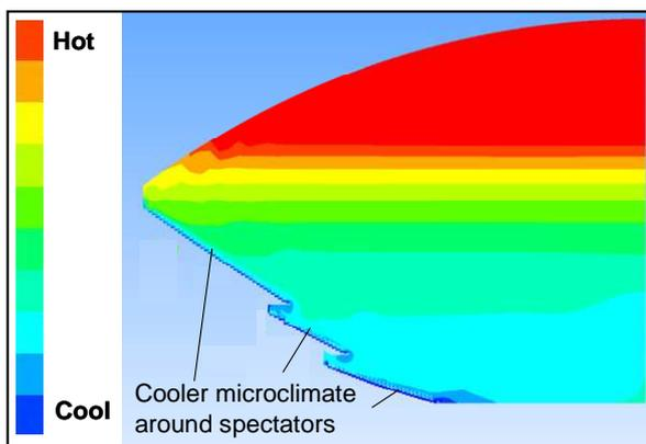
**Figure 3: Under-seat air cooling system creating a local microclimate around spectator zone**
