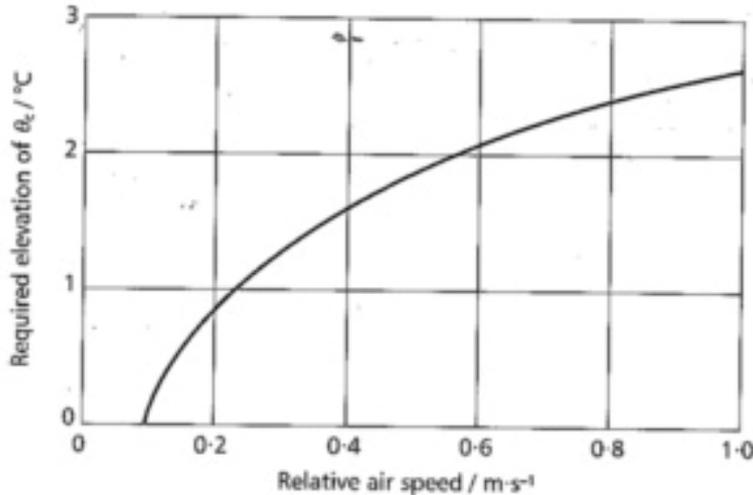
Figure 1.1 Correction to operative temperature ( $\theta_o$ ) to take account of air movement
