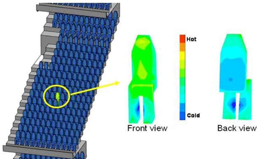
**Figure 5: CFD predictions of operative temperature "next to the body"**
