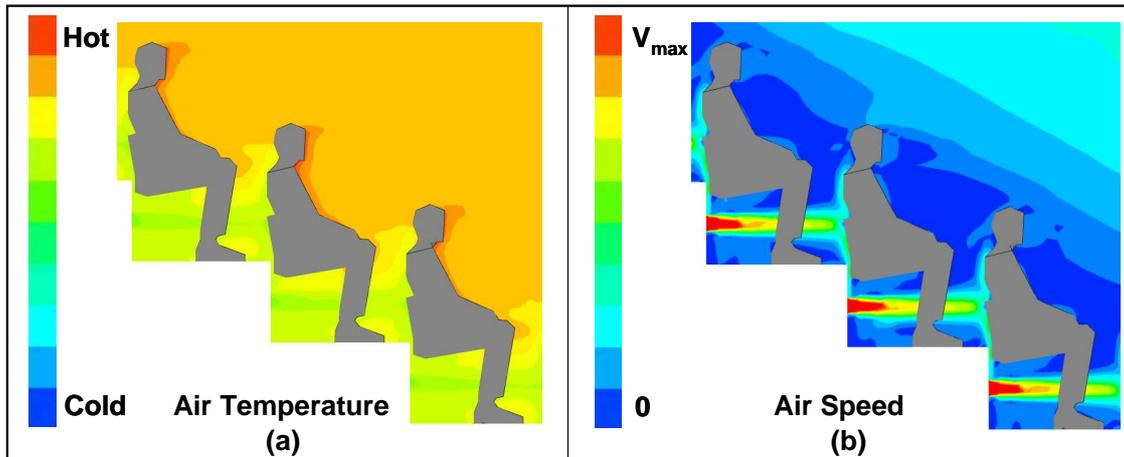
**Figure 4: CFD predictions of (a) air (dry bulb) temperature and (b) air speed**
