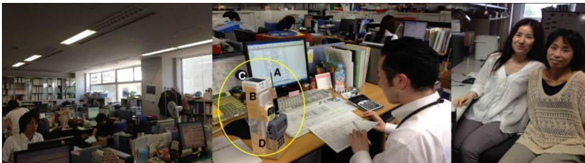
Figure 1. Typical survey environments, measurement setup and typical female clothing ensembles; (A) Omnidirectional probe anemometer (Kanomax Climomaster 6531), (B) Thermo-hygro-CO 2 meter (TR-76Ui), (C) Globe thermometer (TR-52i)
