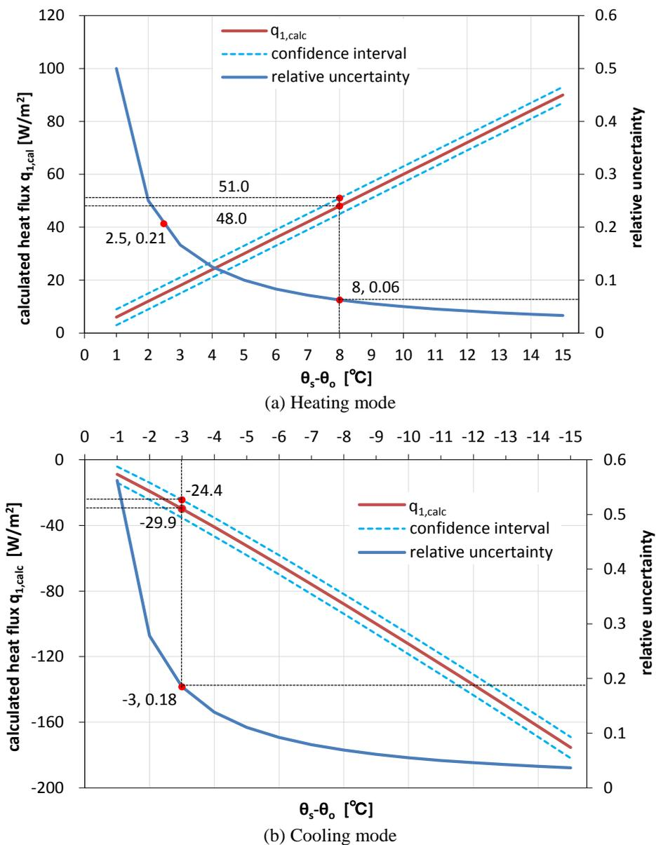
Figure 9 Relative uncertainty of calculated heat flux  $q_{1,calc}$
