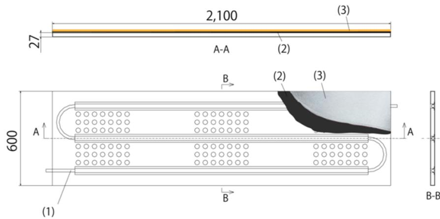
(1) Polybutene pipe (2) Aluminum board (3) Insulation board
