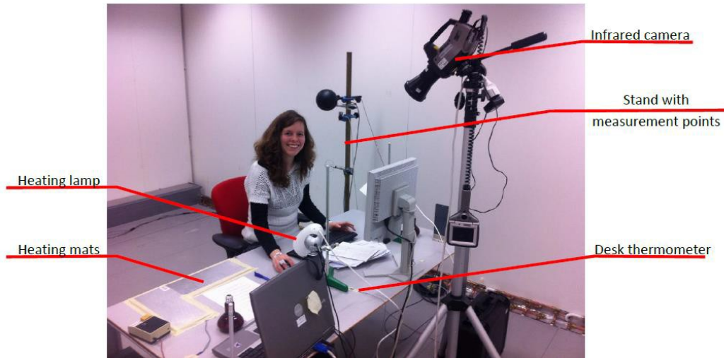
Figure 6: test set up in the climate chamber
