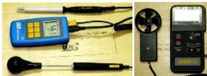
Figure 2a. Temperature Probes and Anemometer
