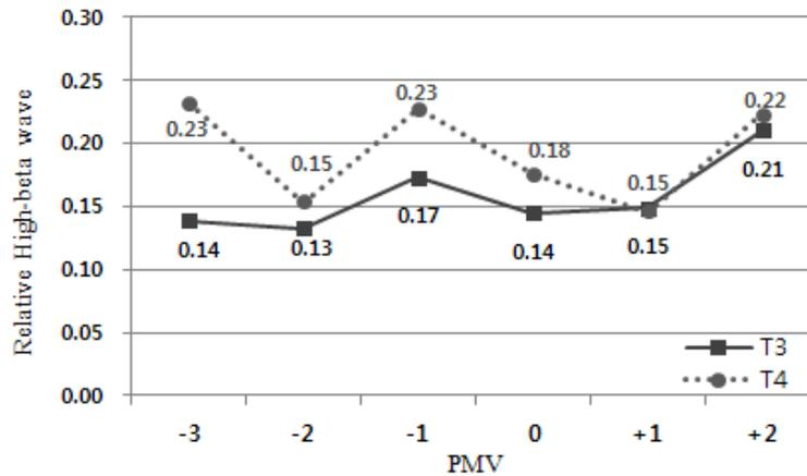
Figure 6. Relative High-beta wave in the temporal lobe based on PMVs (between 63~65 minutes)
