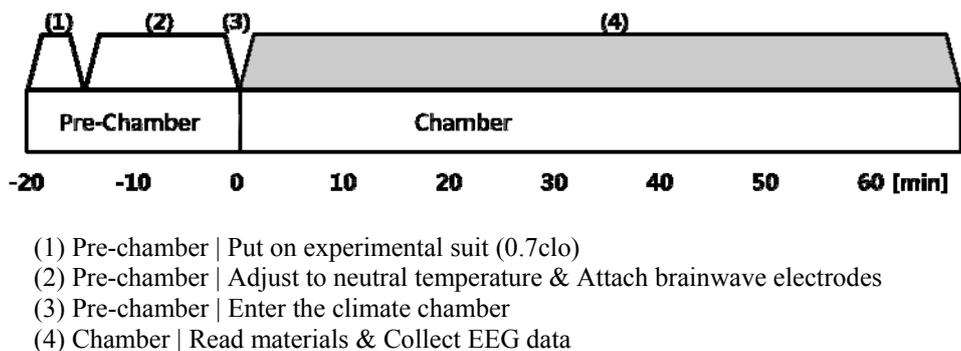
Figure 2. Experimental procedure
