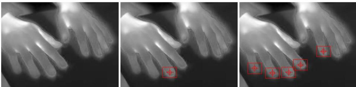
Figure 1 Pattern matching in a static image (from left: source image, marked pattern, matched patterns)
