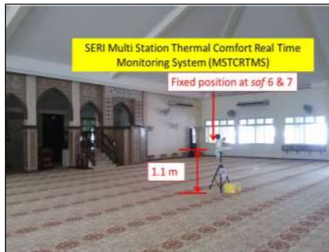
a) Thermal comfort station in MPH
