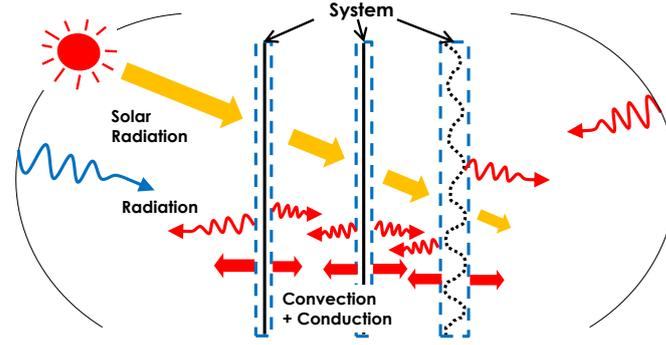
**Figure 2.** Window system consisting of three layers. Each of the layers can be regarded as a thermodynamic system. Whether a system assumed is opaque, transparent, or translucent, some amount of solar exergy is absorbed, consumed, and thereby thermal exergy is transferred to the surrounding space either by the emission of long-wavelength radiation, by conduction, or by convection. The system also absorbs thermal radiant exergy coming from surrounding surfaces.
