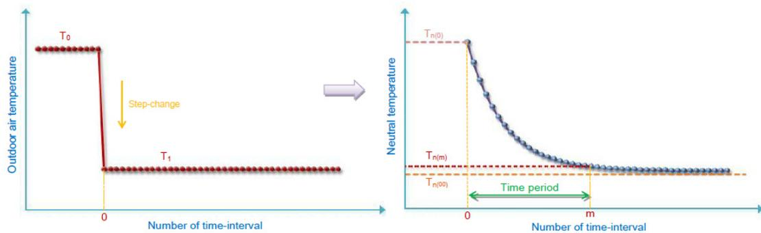
Fig. 1 Definition of time period of thermal adaption. The outdoor air temperature suddenly changed from  $T_0$  to  $T_1$ .  $T_{n(0)}$  is the neutral temperature at the initial time “0”.  $T_{n(\infty)}$  is the theoretical boundary of the neutral temperature during the thermal adaption process.  $T_{n(m)}$  is the neutral temperature at the  $m$ th time-interval.
